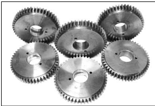
Figure 4: The test gear pairs used in this study. (a) \delta = 0 , ICR = 1.8 , (b) \delta = 10 \mu\text{m} , \delta = 20.9 \text{ deg} , ICR = 1.8 , and (c) \delta = 0 , ICR = 1.4 .
