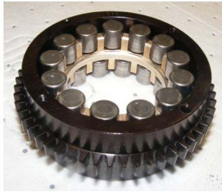
Fig. 8. Experimental planet gear with duplex cylindrical roller bearing. The bearing outer race is the planet gear body, and the inner race is the solid planet pin (not shown).
