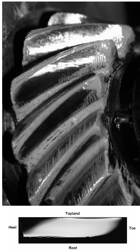
Figure 12. Comparison of the experimental loaded tooth contact pattern (above) with the numerical one (below).
